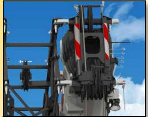
Quick reeve boom head eliminates the need to remove the becket when it becomes necessary to change the reeving.
