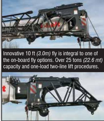
Innovative 10 ft (3.0m) fly is integral to one of the on-board fly options. Over 25 tons (22.6 mt) capacity and one-load two-line lift procedures.
