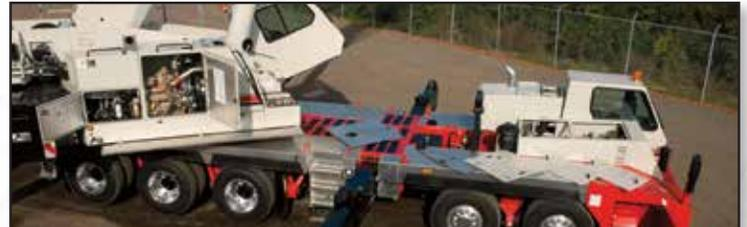
Access to the engine compartments and the operator's cab is superb with strategically-located ladders and steps.
