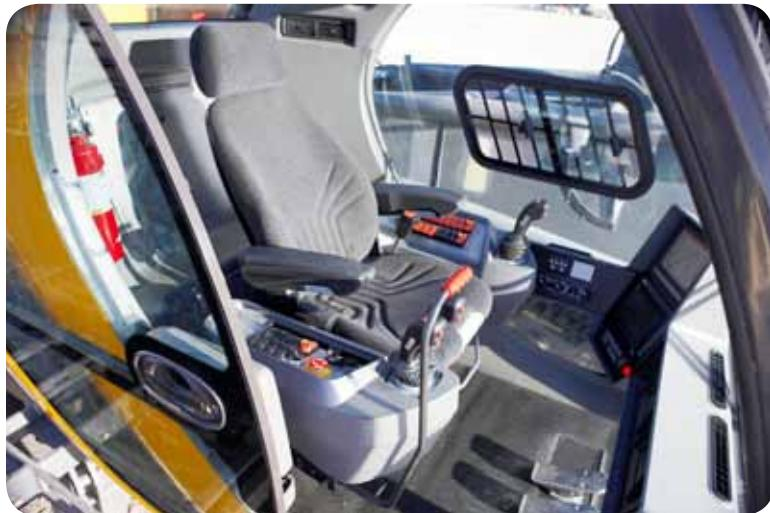
The Operators Cab, designed by Porsche, maximizes glass space for optimal operator visibility and operational safety. The working lights and light bar are standard and well positioned. Equipped with adjustable seats and air conditioner. The cab can be tilted up to a 20° angle and be rotated to the front of platform for transport.
